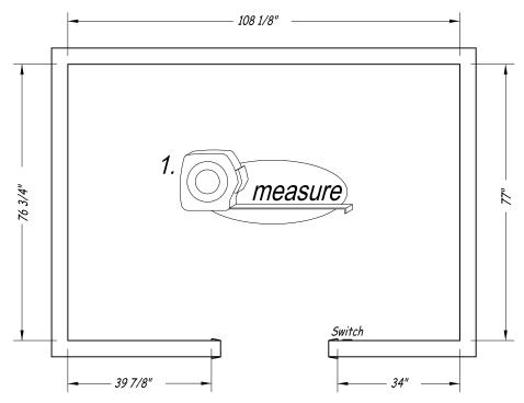
Carefully measure all of the walls and openings around the room. Measure and note all of the items such as light switches, electrical outlets and door casing that must be worked around.
