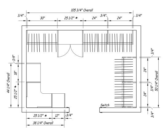
\* When using Corner Units or Door/ Drawer Units please note that those sections include end panels and can share those panels with neighboring sections. Remember to add in all other panel thicknesses for other sections as shown on the example above.
