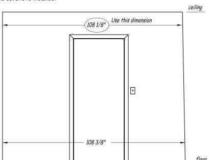
Some walls may be out of plumb or out of square. Be sure to check for such conditions as it may affect your closet system installation. Check room dimensions higher up on the walls in addition to at the floor. Use the smaller of the dimensions.
